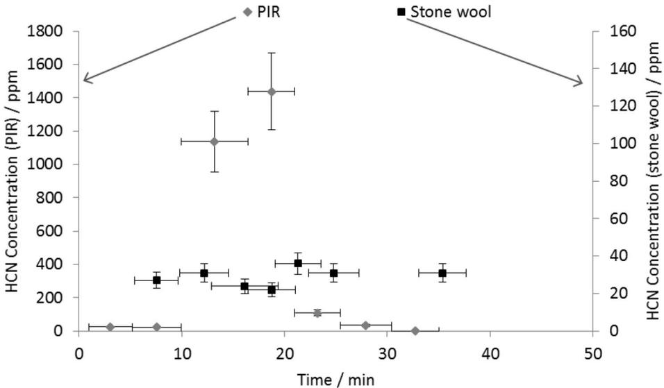
**Figure 17. HCN concentrations—wooden crib experiments (horizontal bars indicate duration of bubbler sampling, vertical bars indicate measurement uncertainty). HCN concentrations from PIR experiment are on the left hand axis, and HCN concentrations from the stone wool experiment are on the right hand axis.**
