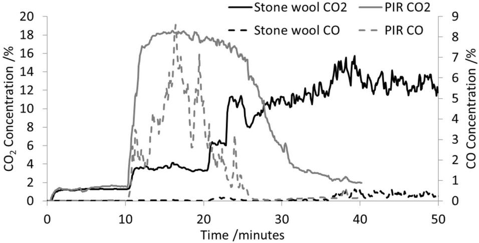
**Figure 16. CO and CO<sub>2</sub> concentration at doorway—burner and wooden crib experiments.**
