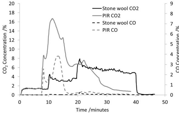
**Figure 9. CO<sub>2</sub> and CO concentrations at doorway—burner only experiments.**
