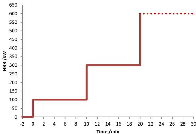
**Figure 3. Planned burner output. The first 20 min are equivalent to the input heat release rate prescribed in ISO 13784-1.**
