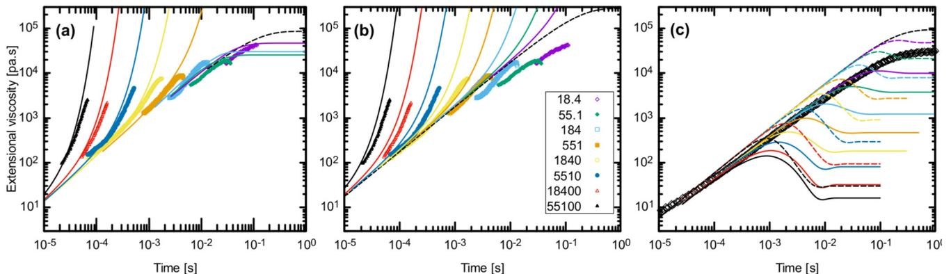
FIG. 12. Comparison of experimental data to the shear and extensional rheology predictions of GLaMM and the Giesekus model with  $\alpha = 0.5$ , showing that the Giesekus model cannot fit all flows simultaneously with a single value of  $\alpha$ . (a) Comparison of GLaMM to experimental extension; (b) comparison of Giesekus to experimental extension; and (c) GLaMM (solid lines) and Giesekus (dotted lines) compared to experimental transient shear.
