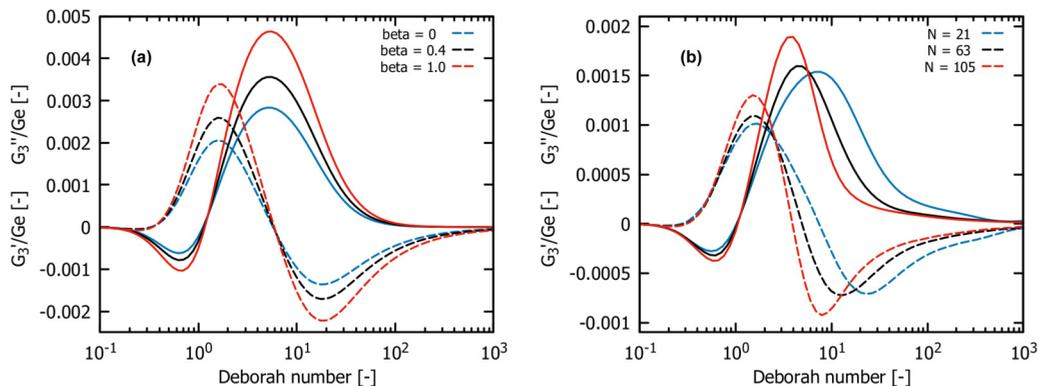
FIG. 10. (a) Variations in the third harmonics as a function of the Rolie-Poly parameter  $\beta \in [0, 1]$ . The amplitude of features in the third harmonic is shown to increase with increasing  $\beta$ , which parametrizes constraint release. Notice that the crossover does not vary with the amount of CCR. (b) The GLaMM third harmonic predictions shown with different discretization  $N = Z, 3Z, 5Z$ . Little difference is seen in the GLaMM predictions with increased numerical accuracy.
