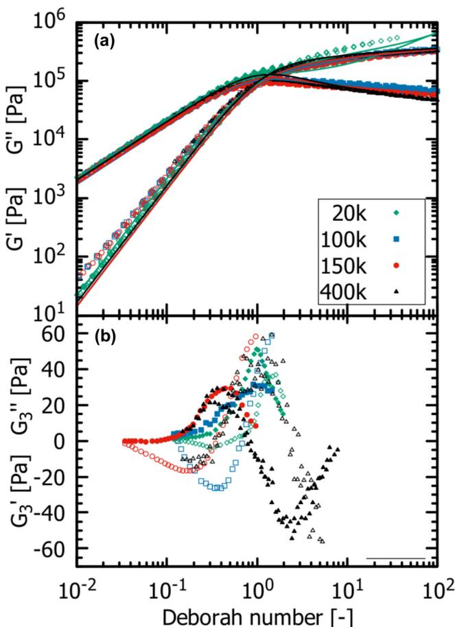
FIG. 6. The analog to Fig. 1 plotted as a function of Deborah number (frequency normalized by terminal relaxation time  $De = \omega\tau_d$ ). The linear rheology superimposes in the terminal region for both theory and experiment.
