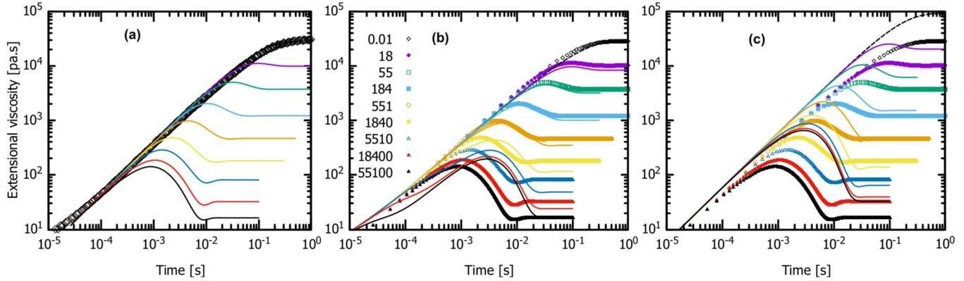
FIG. 9. The shear rheology predictions of the three models used in the main text. (a) The GLaMM model is compared to the linear rheology and the  $\eta^*(t)$  envelope can be observed; (b) the nine-mode Rolie-Poly model is compared to GLaMM predictions; and (c) the one-mode Rolie-Poly model is compared to the GLaMM predictions.
