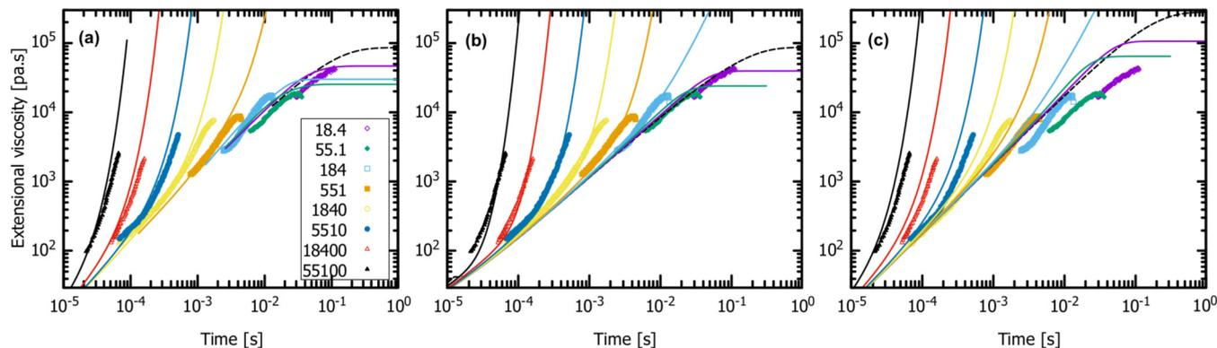
FIG. 8. Extensional rheology measured on a SER attachment at  $-30^\circ$ . Each subpanel compares the extensional data to one of the theories used in the main text: (a) GLaMM, (b) nine-mode Rolie-Poly, (c) one-mode Rolie-Poly.
