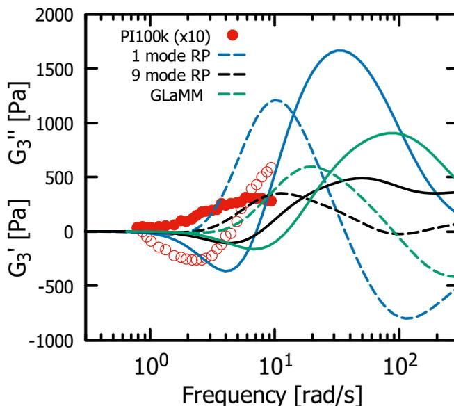
FIG. 3. GLaMM predictions of third harmonics compared to Rolie-Poly with one and nine modes and experimental results. The open symbols and solid lines are  $G'_3$ , and the filled symbols and dashed lines are for  $G''_3$ .
