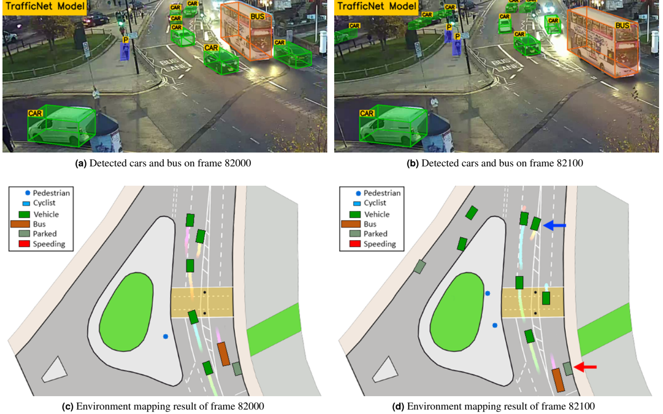
Figure 15. The outputs of adapted 3-head YOLOv5-large algorithm for road-user detection and environment modelling.
