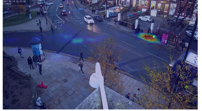
Figure 19. Heat map representation of areas in which vehicles and pedestrians were too close to each other. Source/Location: 10,000 live video frames, Woodhouse lane, Leeds LS2 9JT, UK.
