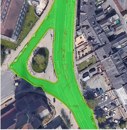
Figure 11. Road segmentation on the satellite image. The red lines represent the initial segmentation result extracted from the SRG method, and the green region is the final segmentation output after applying the morphological operations.
