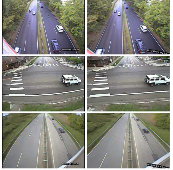
Figure 5. Eliminating the radial distortion in MIO-TCD dataset samples [40]. Left column: original images. Right column: rectified images after barrel distortion removal.
