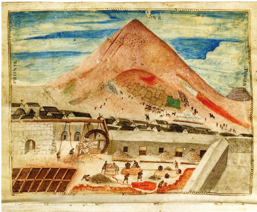
Figure 3. The Cerro Rico with a water-powered stamp mill and amalgamation bins in the foreground, c.1603 (courtesy of the Hispanic Society of America, New York).
