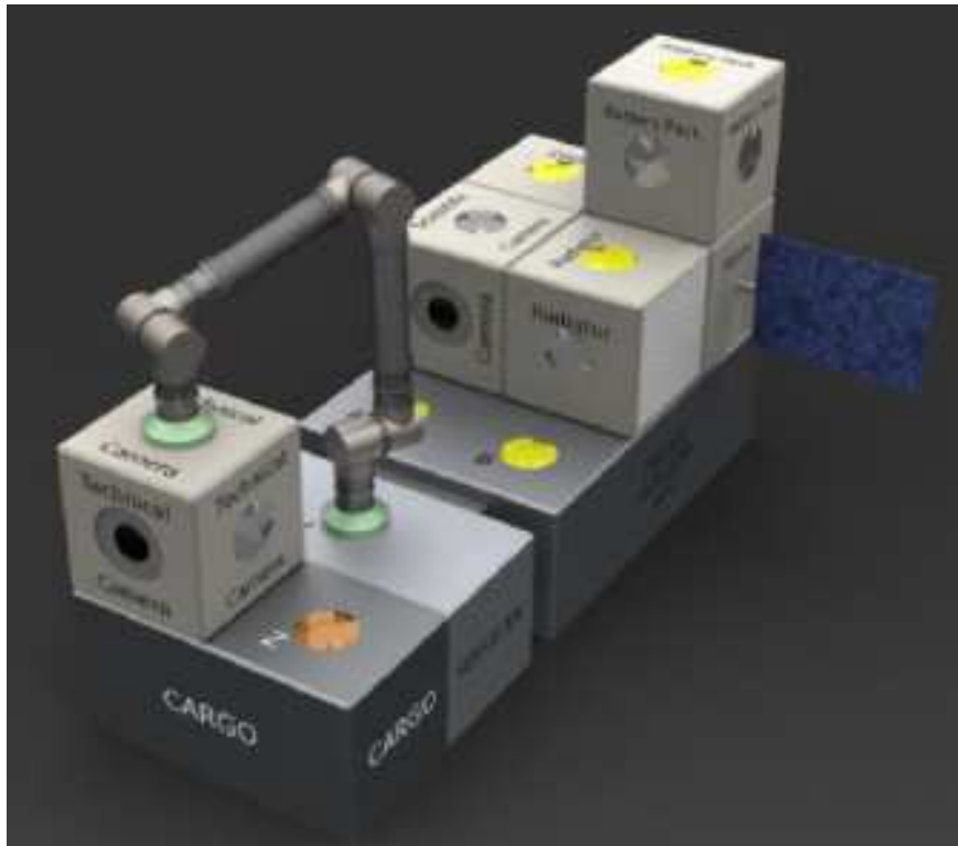
Figure 7. MOSAR Modular Satellite Concept, Space Applications Services NV/SA ( https://www.h2020-mosar.eu )
