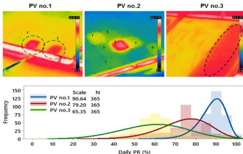
Fig. 5. Calculated PR for three different PV modules affected by different hotpotting conditions.
