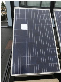
Fig. 6. Opaque paper object covering one solar cell
