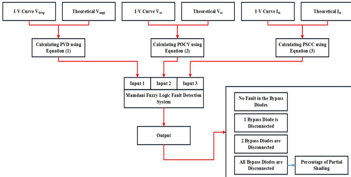
Fig 6: Proposed fault detection system using Mamdani fuzzy logic system
