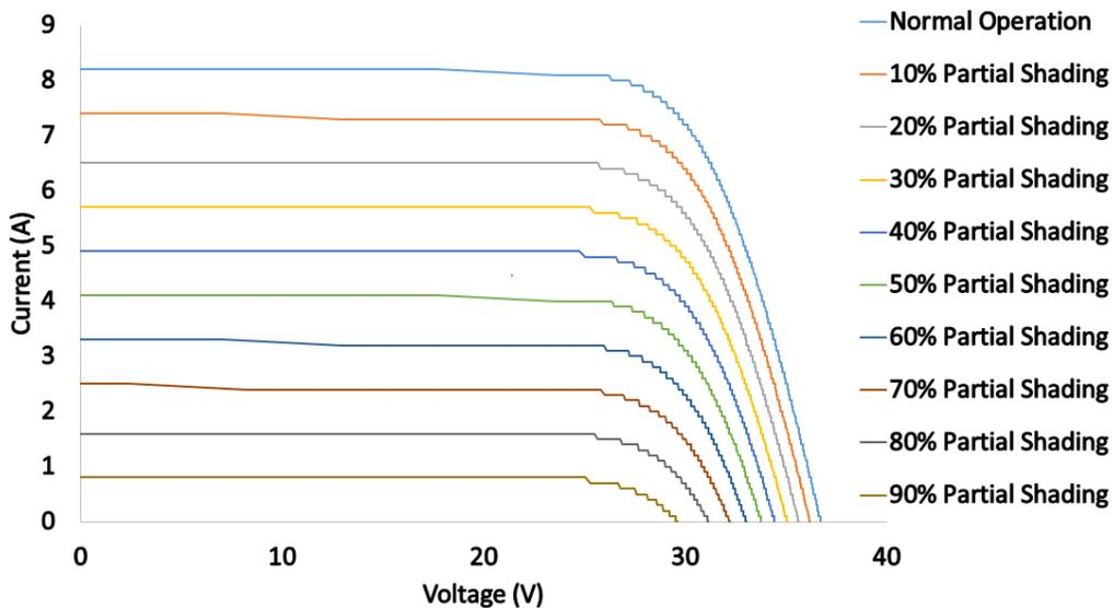
Fig 5: I-V curve simulation under various partial shading conditions while disconnecting all bypass diodes from the examined PV module.
