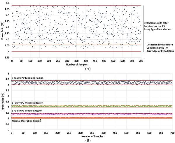
Fig. 13. Power Ratio Variations Obtained by the Second PV System. (A) PR Variations for 3 Faulty PV Modules, (B) PR Variations for all Examined Case Scenarios vs. Detection Limits Which are Explained in Table 4
