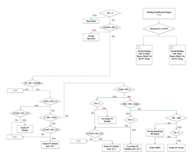
Fig. 6. Diagnosis the error in the DC-Side Faulty Conditions Based on The Voltage and Power Ratios
