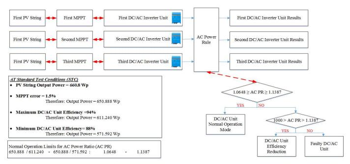
Fig. 7. Diagnosis the Faulty Conditions in the AC-Side Based on Power Ratios
