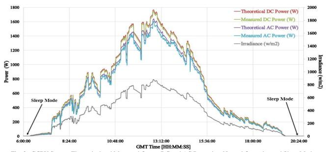
Fig. 8. GCPV System Theoretical and Measured Output DC and AC Power in a Normal Operation and Sleep Mode
