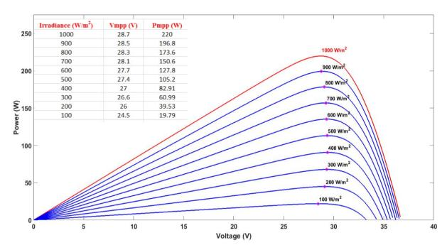
Fig. 3. Power-Voltage (P-V) curve modelling under various irradiance levels
