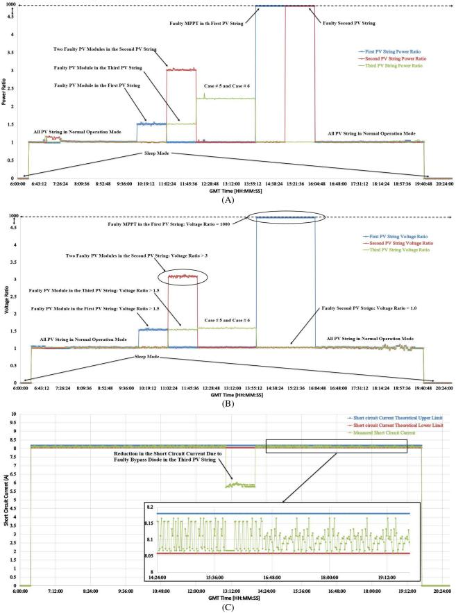
Fig. 11. Diagnosis the Faults Using Fault Detection Algorithm 1. (A) Power Ratio for all PV Strings, (B) Voltage Ratio for All PV Strings, (C) Measured Output Short Circuit Current Variations
