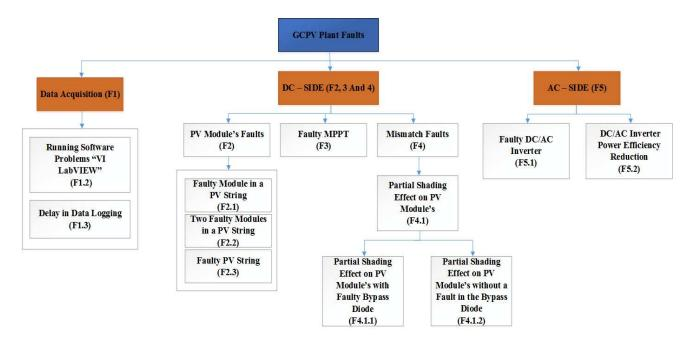
Fig. 1. Different Type of Faults Occurring in the examined GCPV Plant
