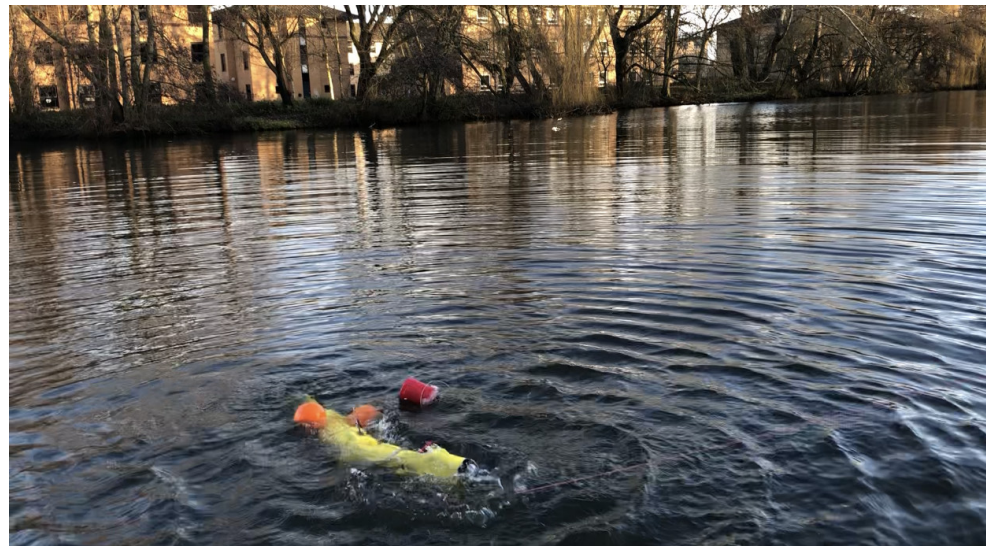
Figure 17. RoboFish prototype swimming on the surface of a lake: two side plastic buoys were included to maintain positive buoyancy; a rope was attached to it to drag it to the home point in the case of failure or battery recharge.
