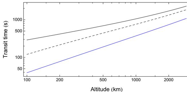
FIG. 8. Transit times (seconds) versus altitudes (kms) for a satellite passing through the zenith in a circular orbit. We plot the total transit time  $t_T$  from horizon to horizon (solid black), the effective transit time  $t_E$  accounting for the mask angle (dashed black) and the quantum transit time  $t_Q$  within the window  $-1 \leq \theta \leq 1$  (solid blue).
