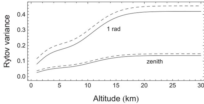
FIG. 15. Rytov variance versus altitude  $h$  (km) for  $\theta = 0$  (zenith) and  $\theta = 1$ , considering  $\lambda = 800$  nm. We plot the Rytov variance assuming the H-V model with night-time parameters (H- $V_{5/7}$  model, solid lines) and the H-V model with typical day-time parameters (dashed lines). In all cases, the Rytov variance saturates at values that are  $< 1$ .
