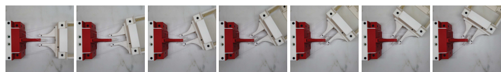
Figure 9. Prototype pitch motion snapshot from 0^\circ to 55^\circ . From left to right the expected angles: 0^\circ, 10^\circ, 20^\circ, 30^\circ, 40^\circ, 50^\circ, 55^\circ .
