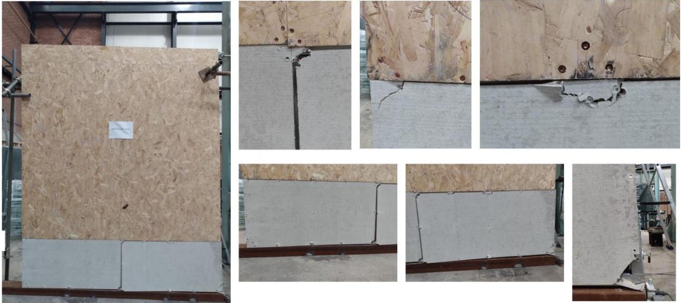
Figure 7. Failure mode of GF walls
