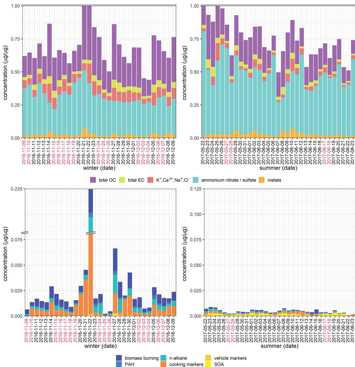
Figure 4. Stacked bar plots of total concentrations for mass-normalised data. OC: organic carbon; EC: elemental carbon; PAH: polycyclic aromatic hydrocarbon; SOA: secondary organic aerosol. “Metals” is the summed concentrations of Al, Ti, V, Cr, Mn, Fe, Co, Ni, Cu, Zn, Cd, Sb, Ba, Pb; “biomass burning” is the summed concentrations of palmitic acid, stearic acid and cholesterol; “PAH” is the summed concentrations of naphthalene, acenaphthylene, acenaphthene, fluorene, phenanthrene, fluoranthene, pyrene, benzo(a)anthracene, chrysene, benzo(b)fluoranthene, benzo(k)fluoranthene, benzo(a)pyrene, indeno(1,2,3-cd)pyrene, dibenzo(a,h)anthracene and benzo(ghi)perylene; “ n -alkane” is the summed concentrations of C 24 , C 25 , C 26 , C 27 , C 28 , C 29 , C 30 , C 31 , C 32 , C 33 and C 34 ; “cooking markers” is the summed concentrations of palmitic acid, stearic acid and cholesterol; “vehicle markers” is the summed concentrations of 17a(H)-22,29,30-trisnorhopane (C 27a ) and 17b(H),21a(H)-norhopane (C 30ba ); “SOA” is the summed concentrations of 2-methylthreitol, 2-methylerythritol, 2-methylglyceric acid, cis -2-methyl-1,3,4-trihydroxy-1-butene, 3-methyl-2,3,4-trihydroxy-1-butene, trans -2-methyl-1,3,4-trihydroxy-1-butene, C 5 -alkene triols, 2-methyltetros, 3-hydroxyglutaric acid, cis -pinonic acid, acid, MBTCA, \beta -caryophyllinic acid, glutaric acid derivative, 3-acetylpentanedioic acid, 3-acetylhexanedioic acid, 3-isopropylpentanedioic acid and 2,3-dihydroxy-4-oxopentanoic acid. Dates marked in red indicate partial or total day haze events as described in Shi et al. (2019). Measurement uncertainty values were unavailable for most data types, and for selected dates in the upper plots, the sum of the total mass measurements is slightly more than 1 (i.e. more than 1 \mu\text{g per } \mu\text{g} ); for these dates, the data have been proportionately scaled. It should be noted that the OC measurement in the upper plots incorporates the variety of organic carbon species represented in the lower plots.
