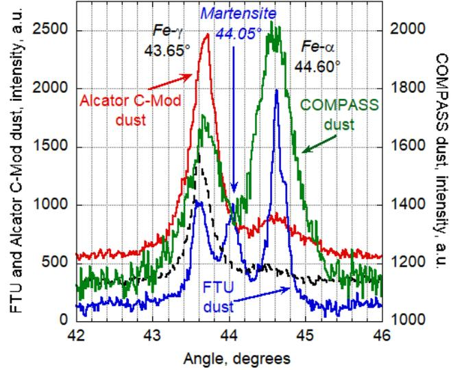
Figure 6: XRD spectra of the Alcator C-Mod (red), FTU (blue) and COMPASS Co4 (green) magnetic dust batches. The spectrum of untreated AISI316 steel is also shown with the black dashed line.
