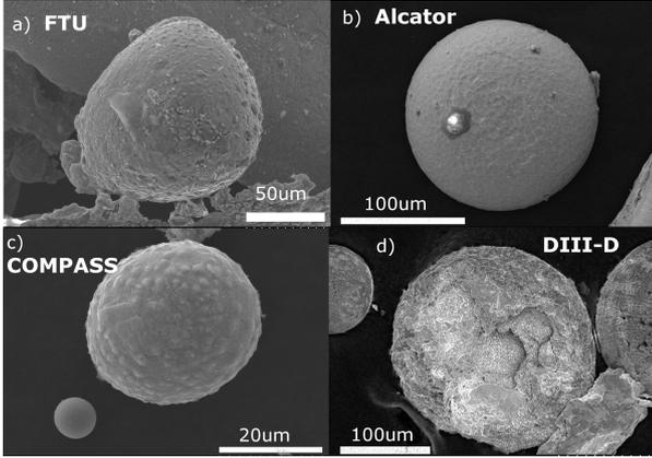
Figure 5: Spheroidal dust *without* any clear dendrite-like textured surface and their EDX analysis (at%). a) SS dust from FTU (C 19.6, O 15.7, Cr 9.6, Fe 47.2, Ni 7.6); b) SS dust from Alcator (C 0, O 0, Cr 21.2, Fe 70.0 Ni 8.0); c) SS dust from the COMPASS Co4 batch (C 50.4, O 9.1, Cr 7.9, Fe 27.4, Ni 4.4); d) SS dust from DIII-D (C 53.4, O 23, Cr 4.7, Fe 15.8, Ni 2.3).
