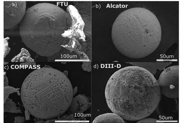
Figure 4: Spheroidal dust *with* clear dendrite-like textured surface and their EDX analysis (at%). a) Ni-based dust from FTU (O 15.4, Cr 12.7, Fe 10.5, Ni 51.24); b) SS dust from Alcator (O 53.7, Cr 8.0, Fe 32.8, Ni 4.8); c) SS dust from the COMPASS Co4 batch (O 48.3, Cr 8.7, Fe 32.1, Ni 3.3); d) SS dust from DIII-D (C 26.9, O 41.6, Cr 7.2, Fe 21.7, Ni 1.9).
