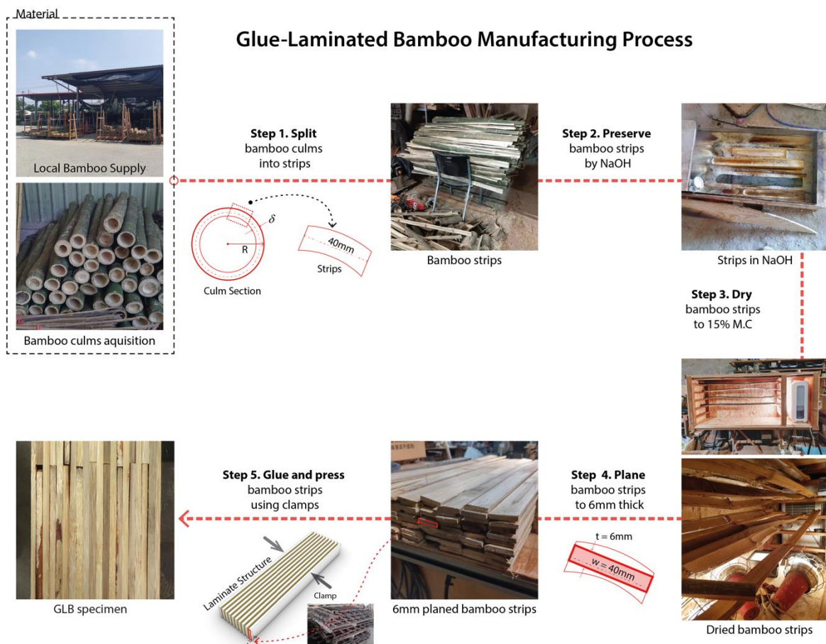
Fig. 2 The manufacturing process of glue-laminated bamboo in Taiwan
