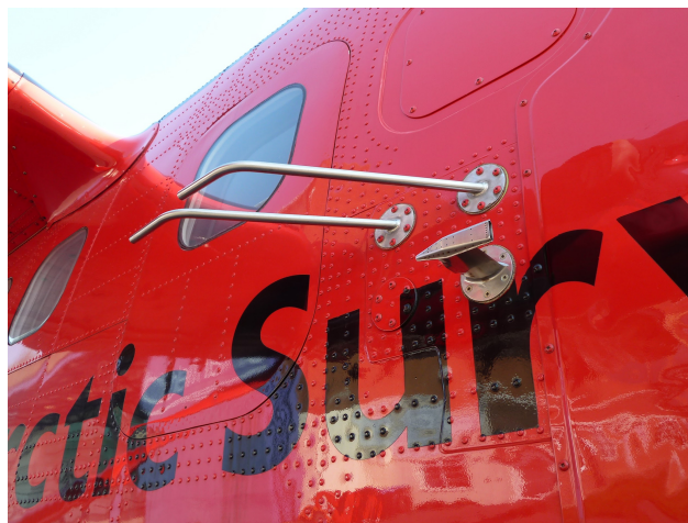
Figure A1. Photo of the rear-facing chemistry inlets on the BAS Twin Otter aircraft.
