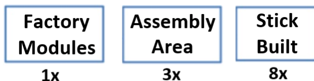
Figure 4 – 1-3-8 rule from shipbuilding (Giovanni Maronati et al., 2018)
