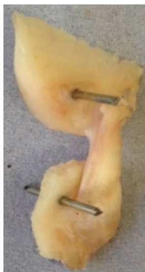
Figure 1: The extracted cranial cruciate ligaments (CCL) consisted of approximately 10 mm of the femoral and tibial bones forming femur-CCL-tibia complex. Two 1.1 mm arthrodesis wires were drilled through the bones to facilitate clamping of the sample.
