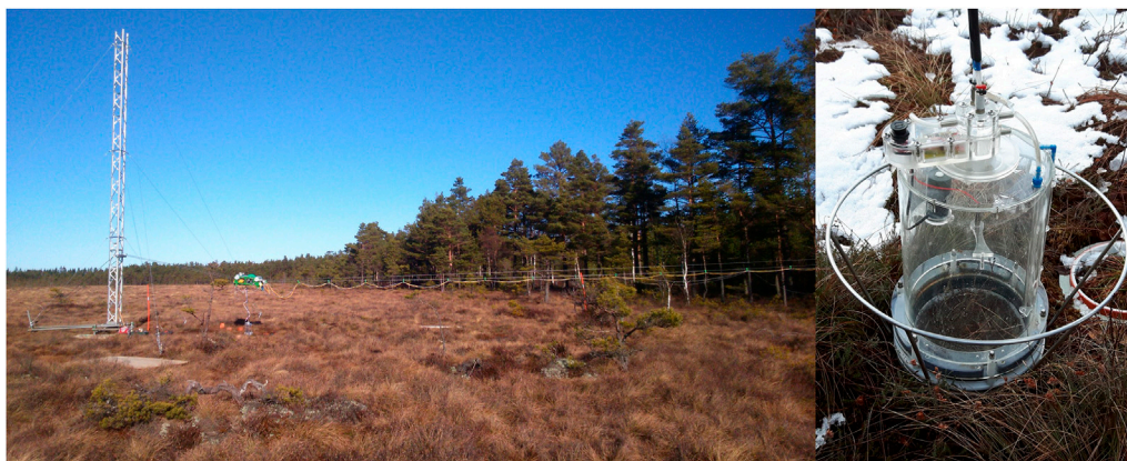
FIGURE 1 | The SkyLine2D system used for GHG measurements at the Mycklemossen field site.
