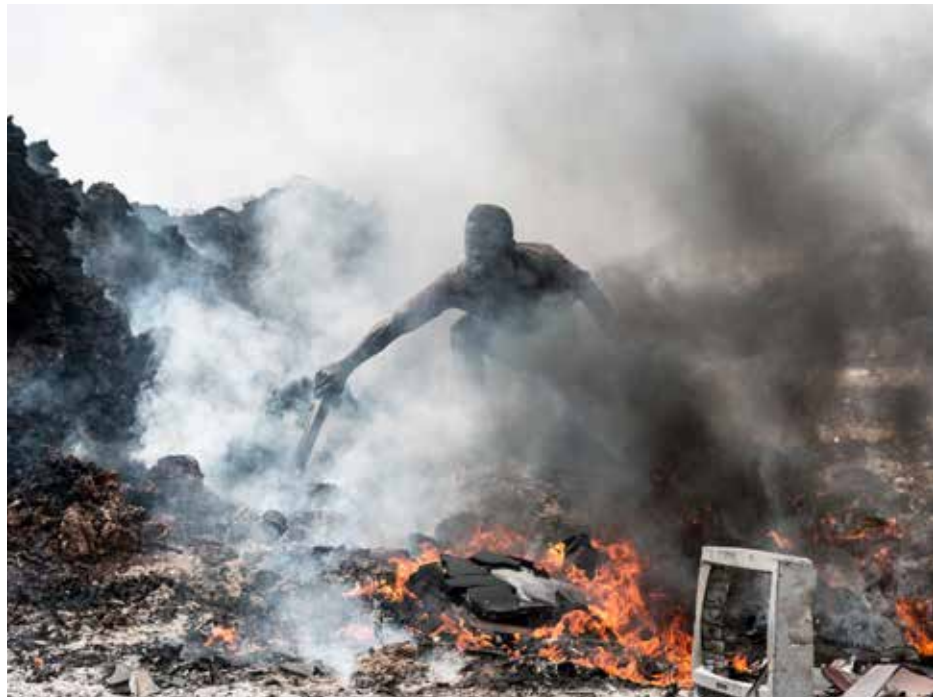
Informal worker recovers metals and components by burning away plastics in Agbogbloshie waste reclamation site, Accra, Ghana; © Aline Tong (2016).
