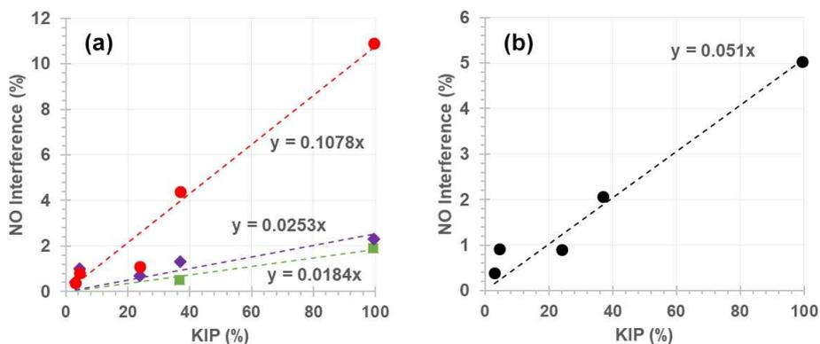
**Figure 5.** Relationship between measured NO interference (%) and kinetic interference potential (KIP; %) for monitors 1 (green), 3 (purple), 4 (red) and the average of the observed NO interference across all instruments (black).
