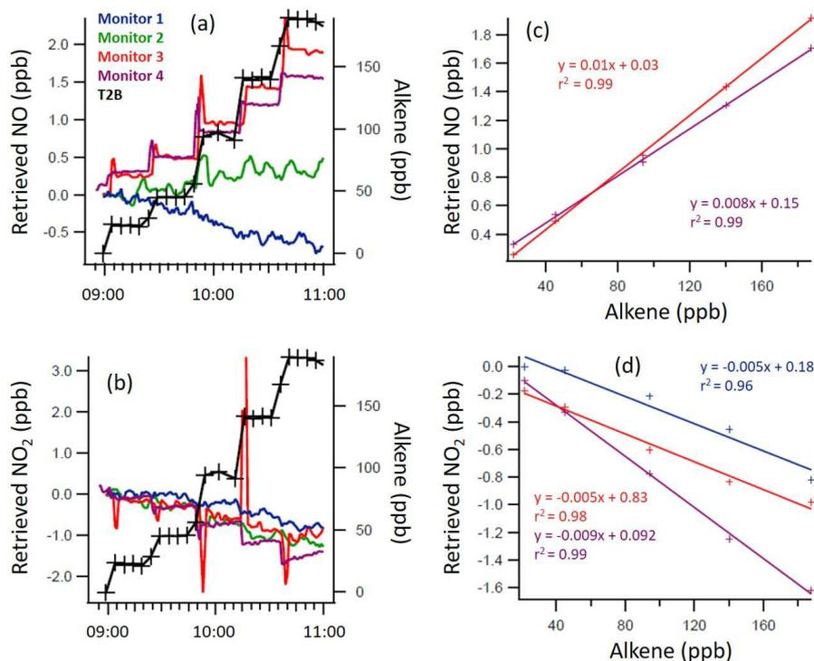
**Figure 4.** Time series of the trans-2-butene (T2B) mixing ratio and measured NO (a, c) and NO<sub>2</sub> (b, d) mixing ratios, as retrieved by each monitor (a, b), with 1 min time resolution, and the regression calculations for the monitors that demonstrated significant interference with the addition of T2B (c, d). Note the different y axis scales.
