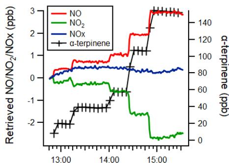
**Figure 6.** Time series of the  $\alpha$ -terpinene mixing ratio (black) and measured NO (red), NO<sub>2</sub> (green) and NO<sub>x</sub> (blue) mixing ratios, as retrieved by monitor 1 (TE42i-TL), with a 1 min time resolution.
