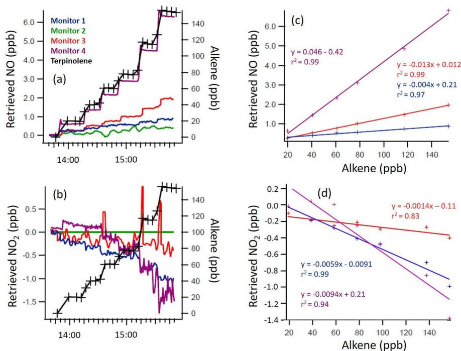
**Figure 3.** Time series of the terpinolene mixing ratio and measured NO and NO<sub>2</sub> mixing ratios, as retrieved by each monitor (a, b), with 1 min time resolution, and the regression calculations for the monitors that demonstrated significant interference with the addition of terpinolene (c, d). Note the different y axis scales.
