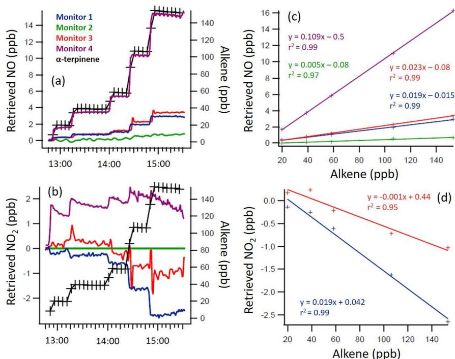
**Figure 2.** Time series of the  $\alpha$ -terpinene mixing ratio and indicated/measured NO (a, c) and NO<sub>2</sub> (b, d) mixing ratios, as directly retrieved by each monitor (a, b), with 1 min time resolution, and the regression calculations for the monitors that demonstrated significant interference with the addition of  $\alpha$ -terpinene (c, d). Note the different y axis scales.
