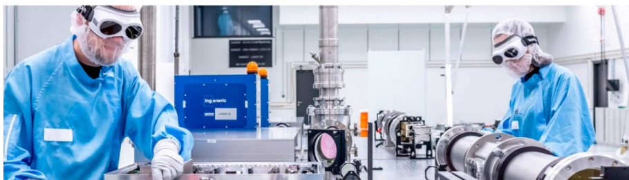
Fig. 29.7. The L2 “Amos” laser system is under development now at ELI-Beamlines (20 J, 10 Hz) (image courtesy of ELI Beamlines).
