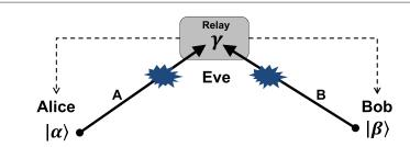
**Figure 1.** Basic protocol of CV-MDI-QKD. Alice and Bob encode information by modulating the amplitude of coherent states, which are sent to an untrusted intermediate station. The relay detects the incoming signals by performing a Bell measurement whose outcome  $\gamma$  is broadcast to the parties. The knowledge of  $\gamma$  allows Alice and Bob to determine the amplitude of the other honest party, by post-processing  $\gamma$  and the amplitudes ( $\alpha$  and  $\beta$ ) in their hands.
