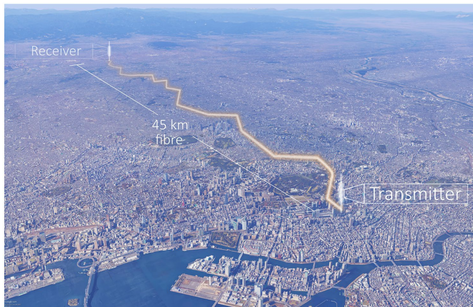
Figure 4. Location of the field trial of the QKD system, with the transmitter sited in central Tokyo and the receiver towards the western edge of the city. The two locations are connected by an installed telecom fibre pair with a length of 45 km and loss of 14.5 dB. Map data courtesy of: Google Earth, SIO, NOAA, U.S. Navy, NGA, GEBCO, Image Landsat and Japan Hydrographic Association.
