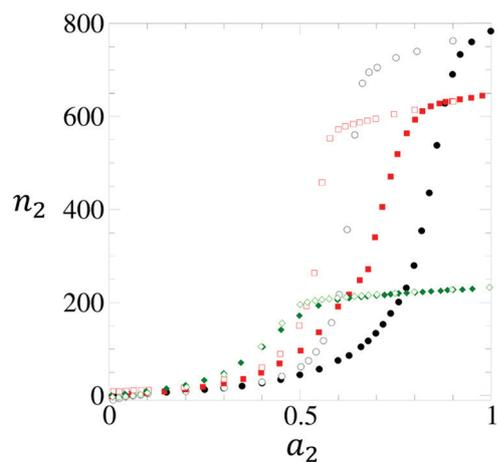
Fig. 2 Adsorption (filled) and desorption (open) isotherms of water vapour on hydrophobic activated carbon fibres, measured by Nakamura *et al.*<sup>68</sup> The pore sizes were 1.1 nm (black circles), 1.0 nm (red squares) and 0.6 nm (green diamonds).
