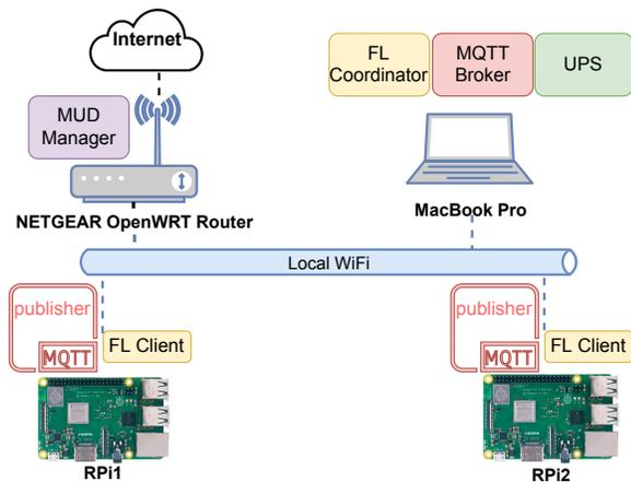
Figure 3: Experimental setup.
