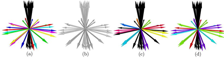
**Fig. 4.** From left to right: (a) vectors from six Lego with ground truth groupings; (b) vectors with no groupings (input to DBSCAN); (c) vector groupings after euclidean displacement or cosine distance DBSCAN; (d) vector groupings after Angular DBSCAN.  $\epsilon = \frac{\pi}{20}$ . Each colour represents a cluster.
