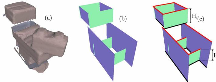
**Fig. 8.** From left to right: (a) input mesh; (b) identified 2x2 brick columns composed of two green and two purple planes each; (c) red and black edges indicate the maximum and minimum y coordinates of each plane,  $H_0$  and  $H_1$  are the distances between the minimum of the maxima y coordinates and the maximum of minima y coordinate of each column.
