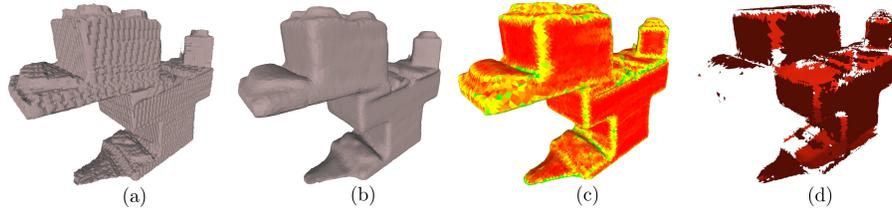
**Fig. 3.** Left to right: (a) input without any smoothing; (b) input after a Laplacian smooth; (c) mesh differentiation with yellow indicating areas of high curvature, and red indicating areas of low curvature; (d) groups of flat surfaces.
