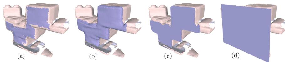
**Fig. 6.** From left to right: (a) input mesh with flat surface; (b) dilated flat surface against mesh; (c) flat surface projected to the identified axis  $A_i$ ; (d) flat surface bounding box projected to  $A_i$ .
