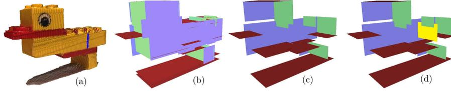
**Fig. 7.** From left to right: (a) input mesh with detected seam superimposed in blue; (b) extracted faces from input mesh; (c) inside of extracted faces, showing no internal face; (d) extracted hidden face highlighted yellow.
