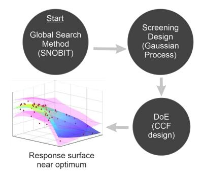
Figure 2. Simplified flow diagram for the hybridised optimisation algorithm.
