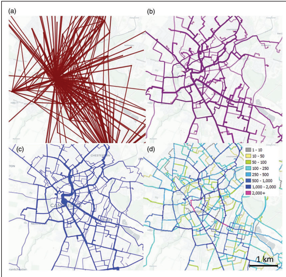
Figure 2. Examples of visualisation of OD data in the PCT and methods of representing number of cyclists: (a) desire lines with thickness proportional to flow, (b) routes with line thickness proportional to flow and using transparency to highlight overlapping routes, (c) aggregated routes into a vector route network, and (d) raster route network with colours representing flow. Base map and data from OpenStreetMap and OpenStreetMap Foundation.
