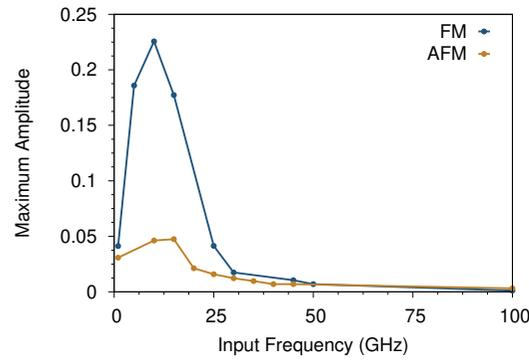
FIG. 5. Comparative plot of the peak power spectral density for the FM and for the AFM interface (0nm from the interface) as a function of different input driving frequencies for CoFe/ $\gamma$ -IrMn<sub>3</sub> with 0.05 T driving field.
