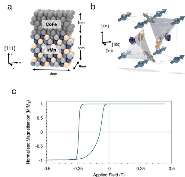
FIG. 1. (Color Online) (a) Schematic diagram of (111) oriented CoFe/ $\gamma$ IrMn<sub>3</sub> bilayer. (b) Simulated ground state magnetic structure of  $\gamma$ -IrMn<sub>3</sub> (c) Simulated hysteresis loop showing exchange bias field arising from an imbalance of sublattice spins at the interface.[16]
