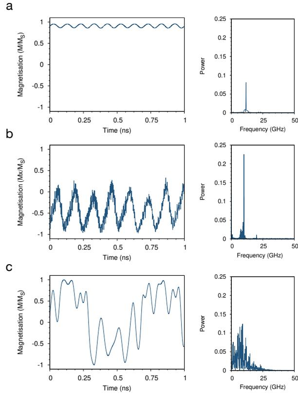
FIG. 3. Response of the ferromagnetic layer to a 10 GHz driving field frequency with an applied field strength of (a)  $B_{\text{fmr}} = 0.01$  T, (b)  $B_{\text{fmr}} = 0.05$  T (c) and  $B_{\text{fmr}} = 0.1$  T. The time data is offset by  $t = 50$  ns after the simulation is started to remove transient effects.
