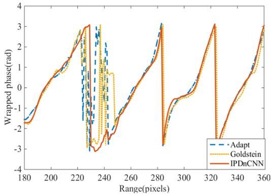
Fig. 17. Cross-sections through denoised phase of airborne data.
