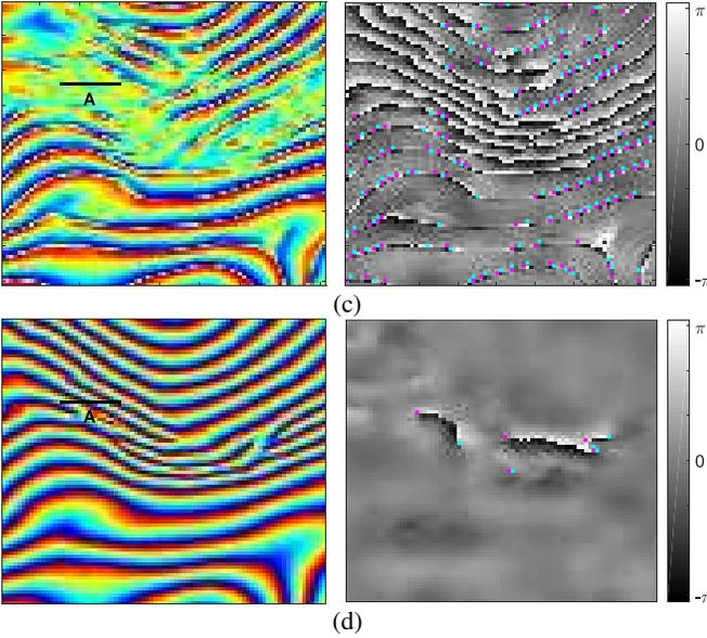
Fig. 9. Denoised phase and phase error: (a) slope adaptive filter with window size  $11 \times 11$ , (b) improved Goldstein filter with window size  $11 \times 11$ , (c) the DnCNN method, (d) the IPDnCNN method.
