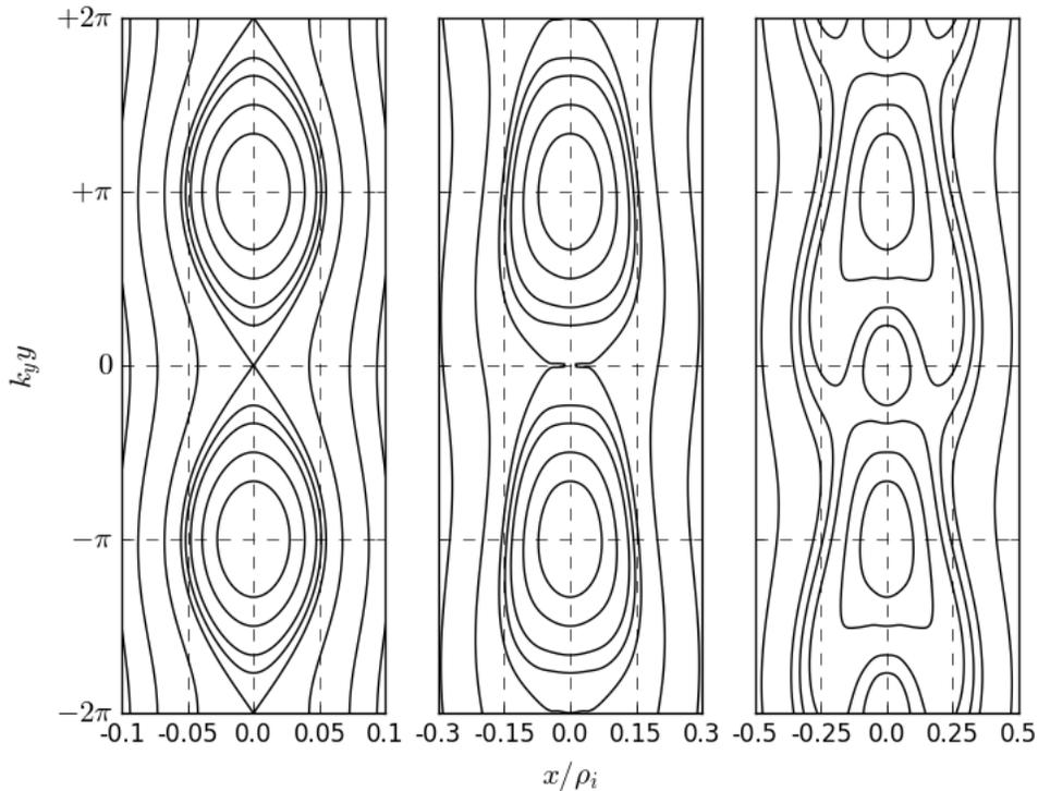
**Figure 9.** The structure of magnetic islands at  $\nu = 0$  growing from small amplitude (left) to large amplitude (right) calculated from our electromagnetic model. Other related parameters are kept the same as in figure (2).
