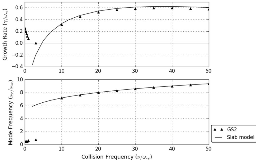
**Figure 2.** The growth rate (top) and mode frequency (bottom) for microtearing modes as a function of collision frequency. The triangle symbols are GS2 simulation results, while the solid lines are a numerical solution of eigenmode equations provided in reference [5]. The parameters used include  $k_y \rho_i = 0.3$ ,  $\eta_e = 5.0$ ,  $\beta = 8\pi n_0 T / B^2 = 0.005$ ,  $m_i / m_e = 1836$  and  $T_i = T_e$ .
