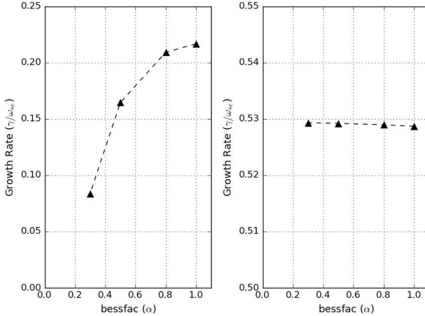
**Figure 5.** The effect of the Bessel factor  $\alpha$  on the collisionless instability (left panel,  $\nu / \omega_{*e} = 0.1$ ) and the collisional MTM (right panel,  $\nu / \omega_{*e} = 20$ ). Other parameters are kept the same as for figure (2).
