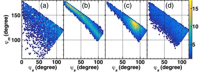
FIG. 3. Two-dimensional plot for a ( $p, 3p$ ) reaction of the two smaller angles  $\varphi_s$  and  $\varphi_m$  in the plane perpendicular to the beam axis. (a) Experimental data for  $^{81}\text{Ga}(p, 3p)$  (b) pair breakup model (c) pair knockout model (d) sequential model. Theoretical distributions have been normalized to the data.
