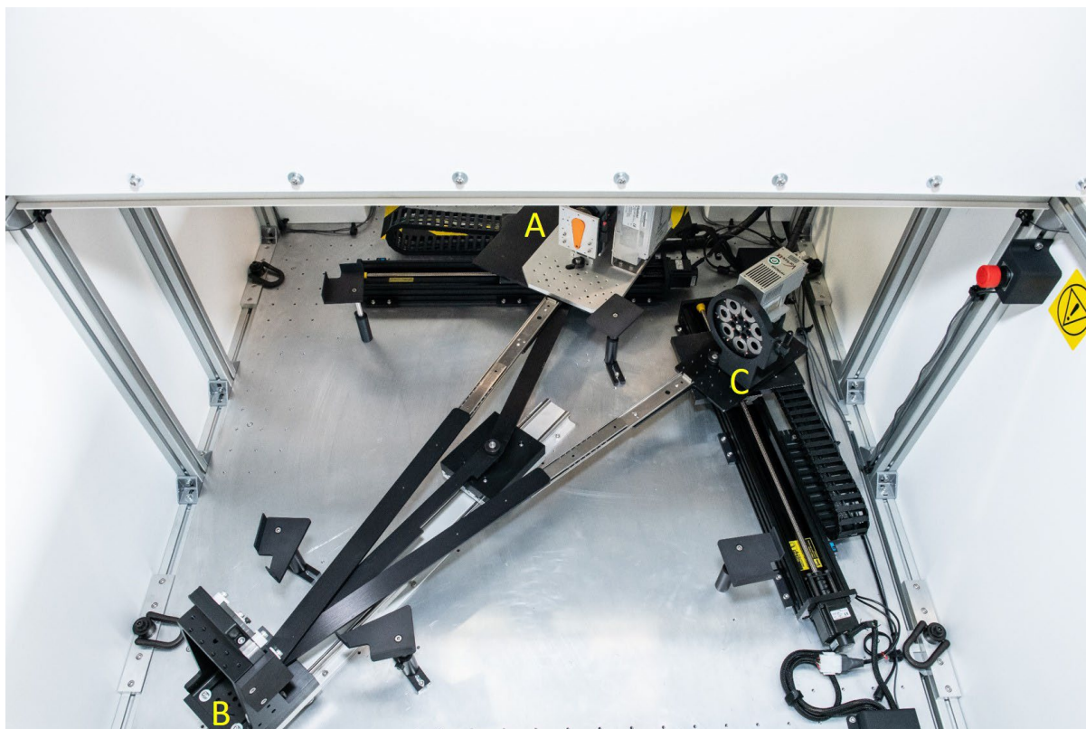
Fig. 2 Photograph of EasyXAFS XES100 spectrometer arrangement shown in Fig. 1, with helium filled beam path removed, to show linear translation stages and steering bars used to maintain alignment of X-ray source (A), spherically bent crystal analyser (B); and sample, slit and detector assembly (C).
