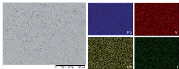
Fig. 12 BSE SEM image at  $\times 2000$  magnification (scale bar length = 30  $\mu\text{m}$ ) and EDX map of Pb (blue), V (red), Pd (yellow), and I (green) present in "PdPb<sub>9</sub>(VO<sub>4</sub>)<sub>6</sub>I<sub>2</sub>" HEBM reacted at 200 °C for 1 h in a sealed quartz tube. EDX spectra are shown in Fig. S2.†
