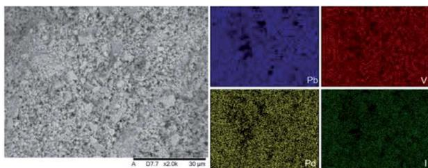
Fig. 7 SEM-BSE image ( $\times 2000$  magnification) and accompanying EDX elemental distribution plots for Pb, V, Pd, and I of batched powders of  $\beta\text{-Pb}_3(\text{VO}_4)_2$  and  $\text{PdI}_2$  subjected to HEBM after 30 h. Scale bar shown at bottom of SEM image represents 30  $\mu\text{m}$ . EDX spectra are shown in Fig. S2.†
