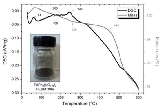
Fig. 9 DSC (black line) and TGA (grey line) curves from 30 to 600  $^\circ\text{C}$  under flowing  $\text{Ar}(\text{g})$  of " $\text{PdPb}_9(\text{VO}_4)_6\text{I}_2$ " batched powders after 30 h HEBM. Insert: resulting powder after 30 h HEBM.
