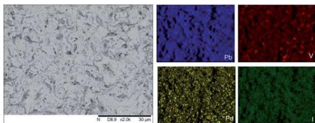
Fig. 13 BSE SEM image at  $\times 2000$  magnification (scale bar length = 30  $\mu\text{m}$ ) and EDX map of Pb (blue), V (red), Pd (yellow), and I (green) present in “ $\text{PdPb}_9(\text{VO}_4)_6\text{I}_2$ ” HEBM reacted at 500  $^\circ\text{C}$  for 1 h in a sealed quartz tube. EDX spectra are shown in Fig. S2.†
