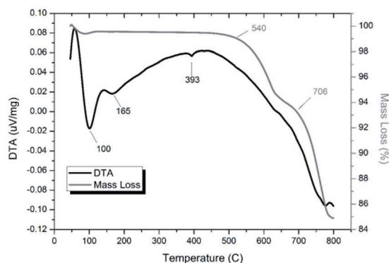
Fig. 14 TGA-DTA analysis of “ $\text{PdPb}_9(\text{VO}_4)_6\text{I}_2$ ” subjected to HEBM 30 h and reacted at 500  $^\circ\text{C}$  for 1 h in a sealed vessel under vacuum.
