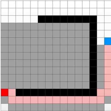
**Fig. 2** The grid cells examined during A\* search from the red square to the blue square. The black squares are an obstacle. The algorithm finds the optimal path from the red square to the blue square but explores a large portion of the grid. The drone would have to fly across all of the grey squares and the pink squares to find the path to the blue square (colour figure online)
