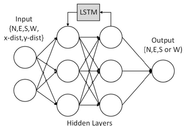
**Fig. 6** Schematic of the PPO and LSTM network. There are 2 hidden layers in our PPO network with 64 nodes per layer. The LSTM provides a recurrent connection between hidden layers. This loop back allows the network “to remember” the previous inputs and to include this recurrent information into the decision-making. Further hyper-parameter settings are given in the “[Appendix](#)”
