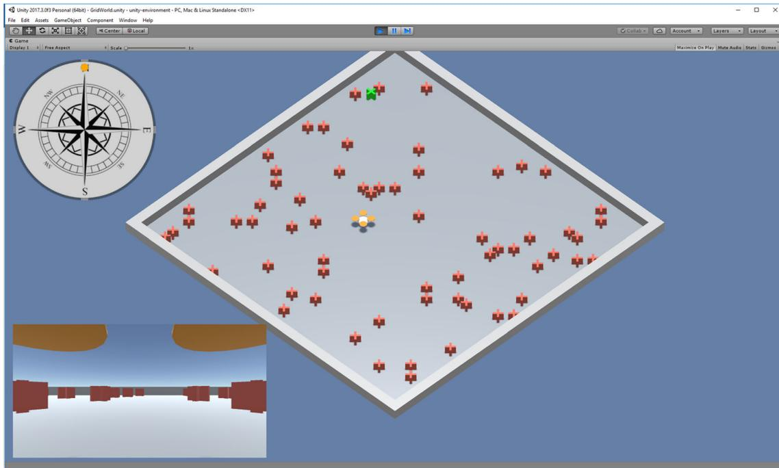
**Fig. 5** A randomly generated Unity 3-D ML-agents Grid-World with a  $32 \times 32$  grid, 64 obstacles (red  $\times$ ) and one goal (green  $+$ ). The AI navigates the drone to the goal. The compass (top left) shows the
