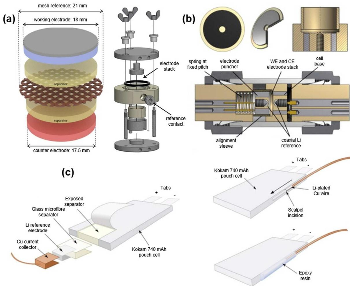
**Fig. 3.** Some of the different three-electrode cell designs: (a) coin cell, where a mesh reference electrode is placed between two separators [23]; (b) coaxial cell developed from a modified Swagelok [24]; (c) commercial pouch cells retrofitted with a third reference electrode [34]. Source: Adapted from references [23,24,34].
