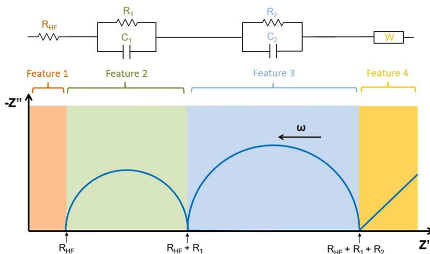
Fig. 2. Schematic idealised impedance complex plane plot for a multicomponent system together with its ideal equivalent electrical circuit.
