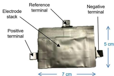
**Fig. 4.** The 10 mAh three-electrode pouch cell used in this study. The reference electrode sits at the top and is sandwiched between two separators, with the cathode and anode either side, inside the cell.
