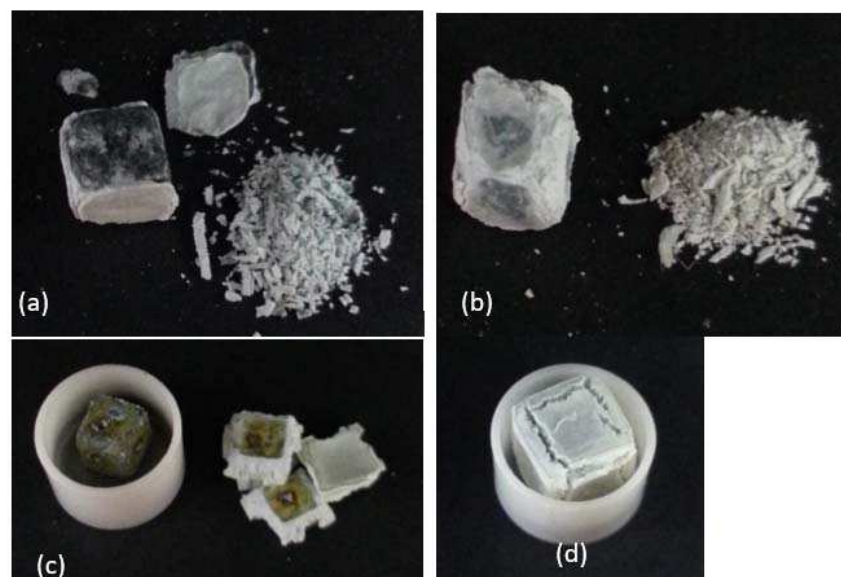
Figure 7. The specimens of the alloys JZ1 (a,c) and JZ2 (b,d) after oxidation at 800 °C (a,b) and 1200 °C (c,d). The size of each oxidation specimen was 3 × 3 × 3 mm 3 .
