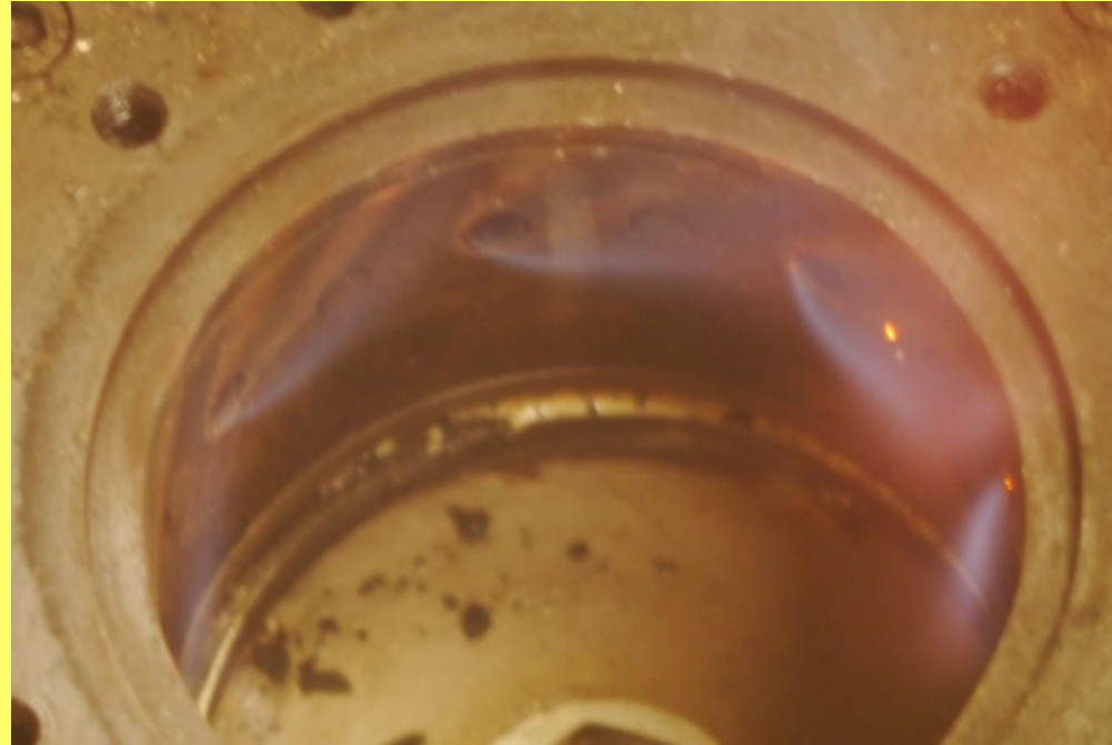
BB, 15.4.19, 15.41 7 kW H 2 \phi = 0.44 Near Invisible flame 839K exit temperature
