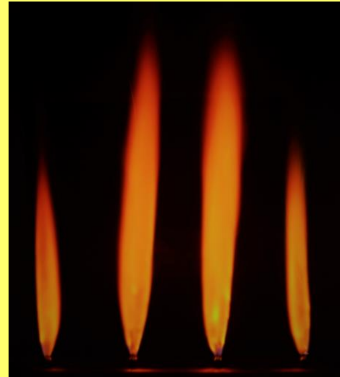
A 4 jet 4 kW burner on H 2
