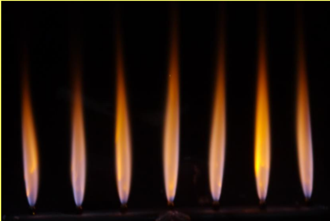
A 7 jet 7 kW burner on hydrogen Note that there is no problem with 'invisible flames'
