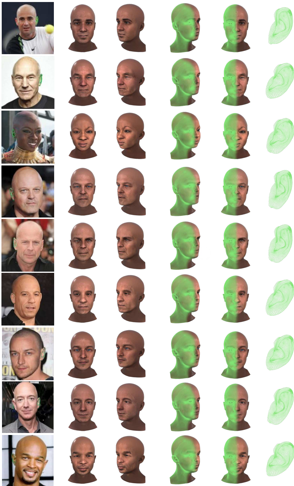
Fig. 13. Qualitative results of our in-the-wild 3D head reconstruction. In the first column we show the 2D ear landmarks on top of the subject images. In columns 2-5 we depict our high detailed head reconstruction. In the last column we illustrate different ear shape reconstructions for each subject. Our model is able to generate realistic representations for all general traits (i.e. face, head, eyes, ears).
