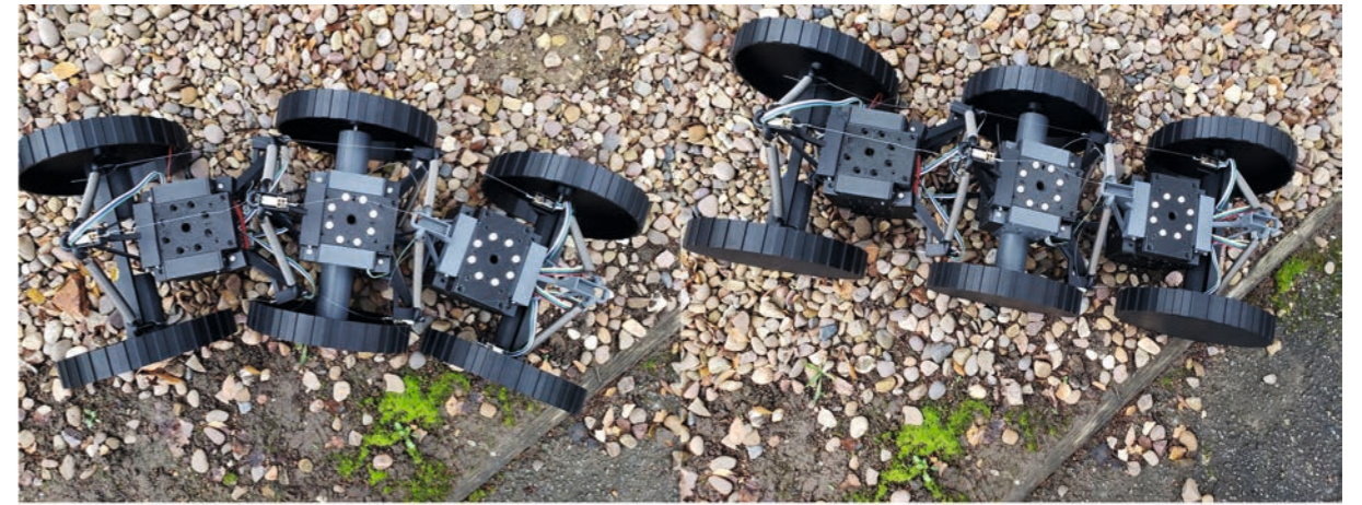
Fig.6 Tensegrity Structure: Example of Structural Programmability. The degree of turning on a slope is determined by varying the stiffness of the tensile elements from compliant (left) to rigid (right).
