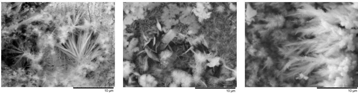
FIGURE 7, XRD OF SAMPLE SURFACES: A) CONTROL SURFACE LEFT IN ROOM CONDITIONS 15 DAYS AFTER RENEWING (TREATMENT A), B) OXIDES SYNTHESISED BY SIMULATION OF TRACKSIDE CONDITIONS (TREATMENT E), C) SURFACE FLOODED WITH 5ML WATER DROP DEPOSITION (TREATMENT F).
