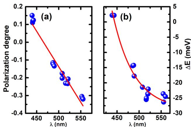
**Figure 3.** (a) Polarization degree as a function of peak emission wavelength; and (b) Energy separation  $\Delta E$  of the two polarized emissions as a function of peak emission wavelength. Solid lines are only as a guide to the eye.
