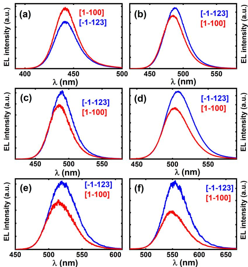
**Figure 2.** Polarized EL spectra measured at 20 mA injection current for the semi-polar (11–22) LEDs with increasing indium content and peak emission wavelength. In each case, the EL spectrum labeled in red was measured at a polarizer angle of  $0^\circ$  corresponding to the electric field aligned along [1–100], while the EL spectrum in blue was measured at a polarizer angle of  $90^\circ$  corresponding to the electric field aligned along [–1–123].
