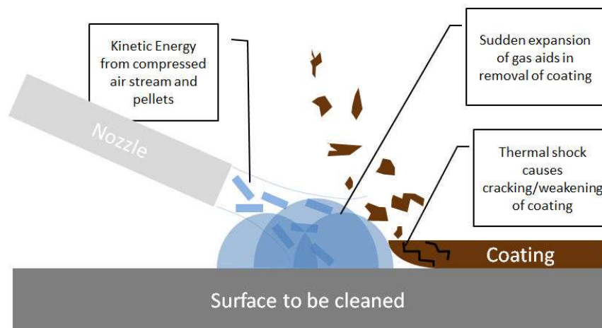
Figure 1. The three mechanisms of dry-ice cleaning
