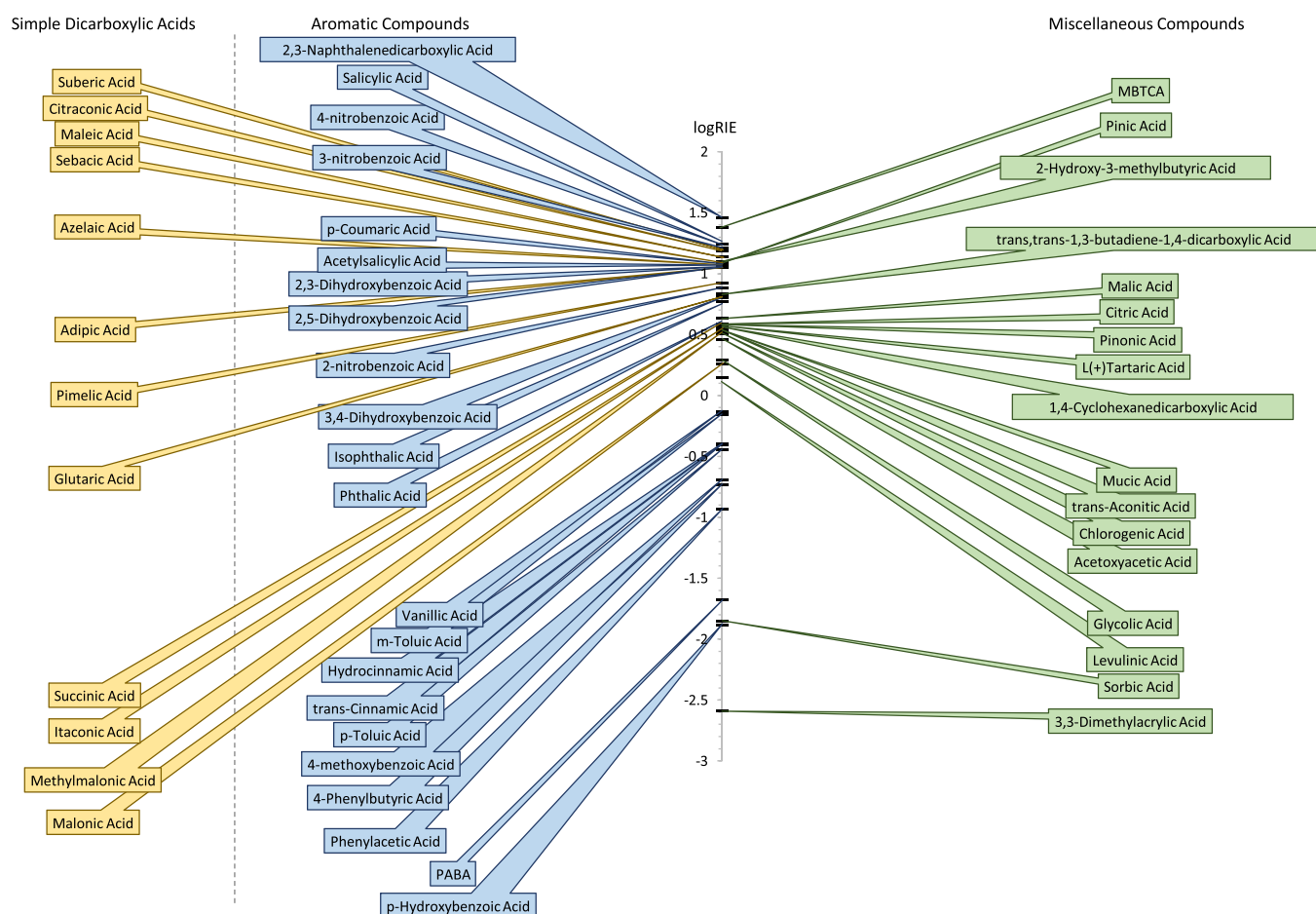
Figure 1. Scale of measured log relative ionization efficiencies (log RIEs), relative to benzoic acid. A table of log RIEs can be found in the Supporting Information, Table S1.
