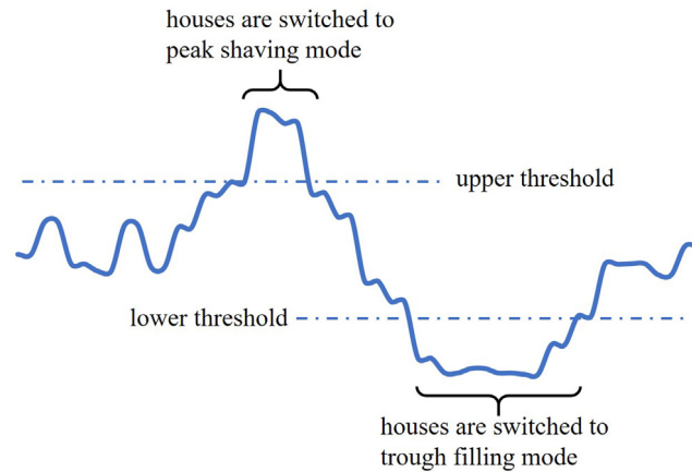
Fig. 3. Illustrates the approach to DSM using two thresholds (the vertical axis is electrical demand).
