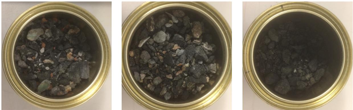
**Figure S3.** Photographs of the three different unprocessed SPL samples selected for leaching trials. Sample A (left), containing a large fraction of cementitious and brick material. Sample B (middle), containing visible cementitious material. Sample C (right), appearing to be mainly graphitic material.
