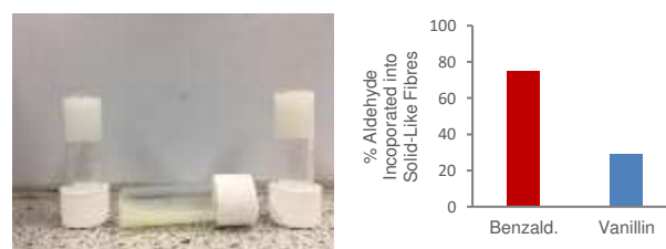
Figure 3. (Left) Photograph of gels formed by (left) 1:1 glutamine amide:benzaldehyde, (middle) 1:1 glutamine amide:vanillin and (right) 1:1:1 glutamine amide:benzaldehyde:vanillin. (Right) Percentage of benzaldehyde and vanillin incorporated into the solid-like gel nanofibres as assessed by 1 H NMR on a gel assembled from 1:1:1 glutamine amide:benzaldehyde:vanillin in D 2 O.
