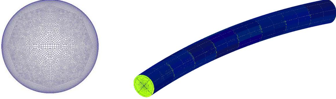
Fig. 1 Cross section and 3D view of the mesh
